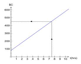
The charge is approximately \$450, accuracy is limited by the size of the graph.
