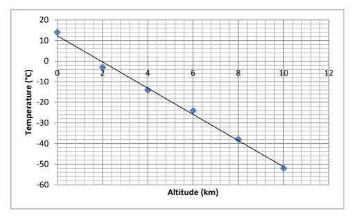
By eye: the y-intercept =12, Using the points (0,12) and (10,-51) the slope is:
