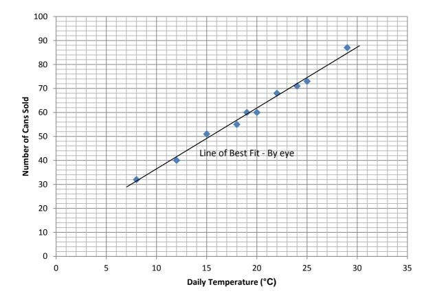
From the scatterplot, there appears to be a linear relationship between the variables. A straight line will not run through every point but a line of best fit can be drawn. There are numerous methods to obtain a Line of Best Fit, three will be given in this module.
